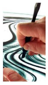
Cutting Glass is an essential skill. The best hand cutting tools today have oil reserves in the handle which helps lubricate the cutting wheel, and penetrates into the the fine fractures caused by the wheel helping it to break evenly.
