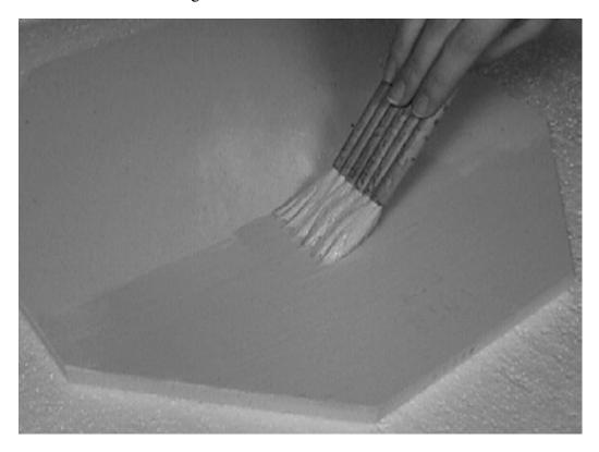
Many coatings will be needed to fully coat the shelf with reasonable drying times between coats. It is possible to hasten the drying process by loading the shelf or mold into the kiln and taking the temperature up to 400 to 500°F.
