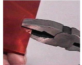
To groze, hold the pliers curved side up and use a rolling motion to gently scrape the glass edge against the serrated teeth. Use the tips in a chewing motion to remove small sections of glass or nibble out deep inside curves.
