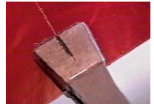
To use, place the jaws (with the center indicator line facing up) squarely onto the glass with the score line centered in the jaws. Turn the adjustment screw until it just touches the bottom handle, then back it off 1/2 a turn. Squeeze the handles gently until the score runs. You must have the jaws fully on the glass for the pliers to work properly.
